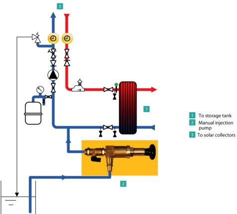
For ease to use, install the top-up pump perpendicular to the wall.
