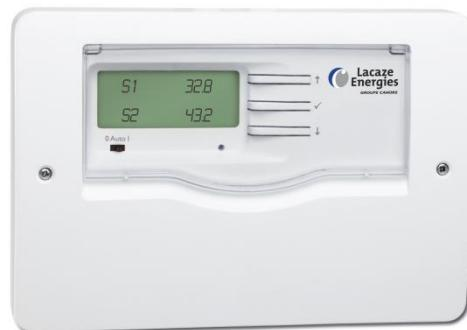
It is usable for all functions of controllers 800X, 600X and 600i. All these functions are set up from the controller. The extension module transmits all the data collected to the solar controller. The temperatures of temperature sensors, the states and the speeds of the relays can be read directly on the module display.
