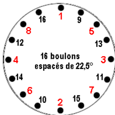
16 bolts spaced at 22.5°
